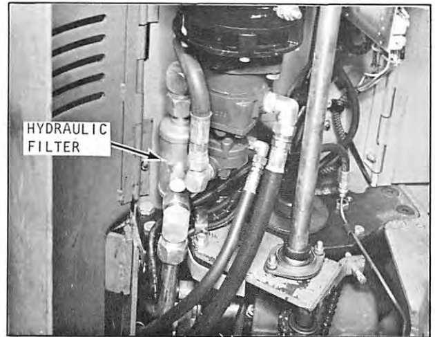
Plate 9491. Typical Hydraulic Filter Hydraulic Filter Location
