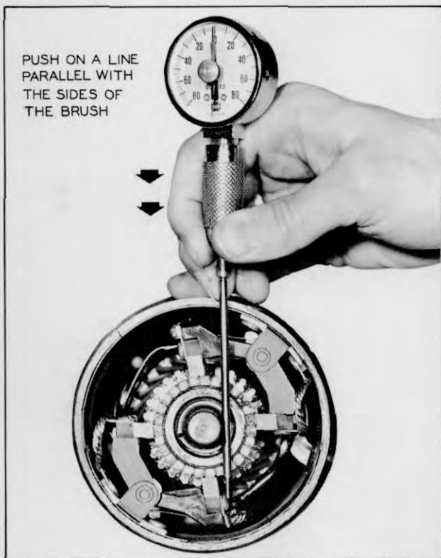
Plate 6449 Checking Brush Spring Tension
