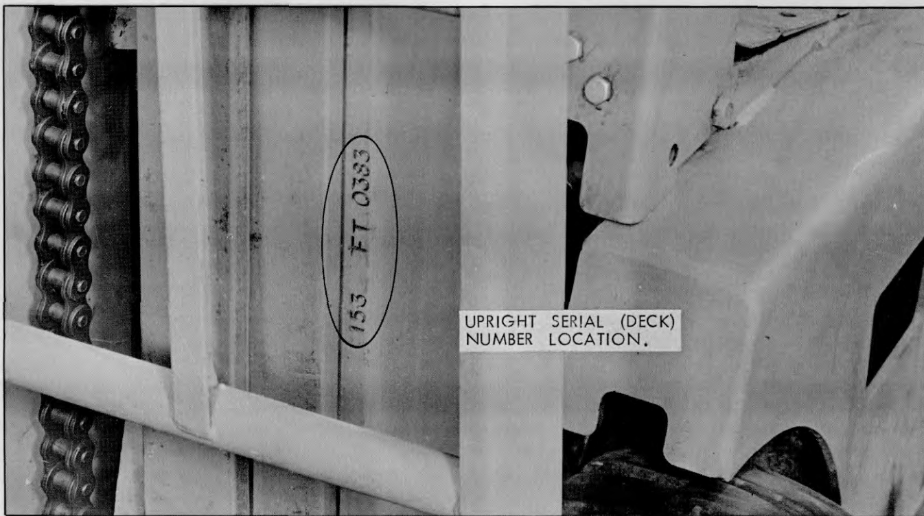
Plate 9475. Upright Serial (Deck) No. Location
