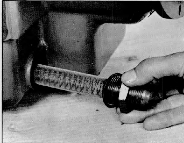
Plate 7235. Transmission Sump Screen
