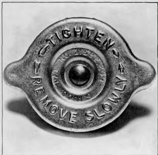
Plate 6458. Radiator Pressure Cap
