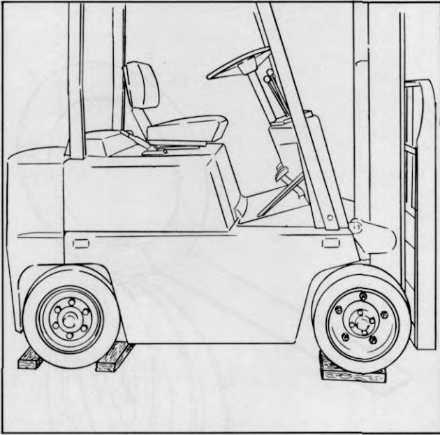
Plate 9811. Drive Wheels on Blocking, Block Steer Wheels
