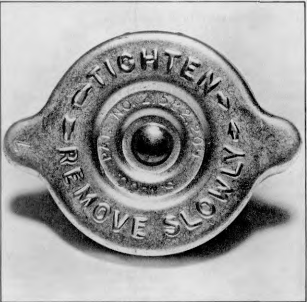
Plate 6458. Radiator Pressure Cap
