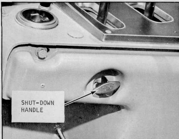
Plate 10178. Typical Shut-down Handle
