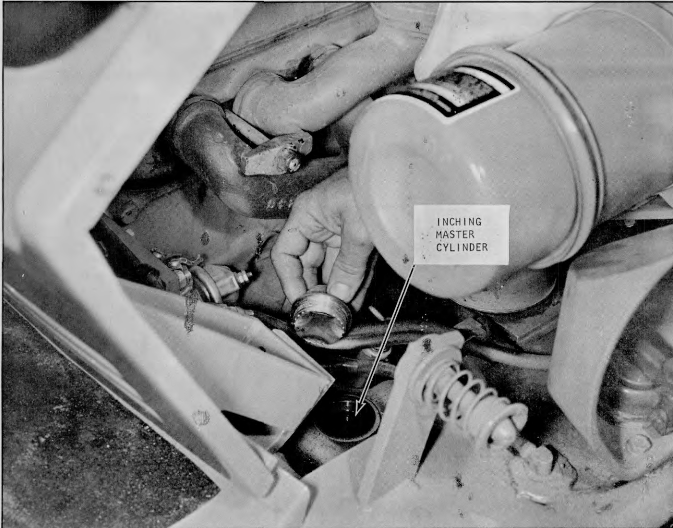
Plate 10182. Typical Inching Master Cylinder
