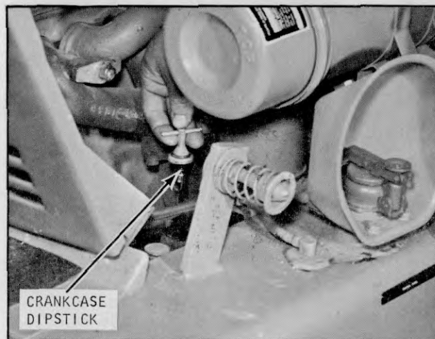
Plate 10186. Typical Oil Level Check
