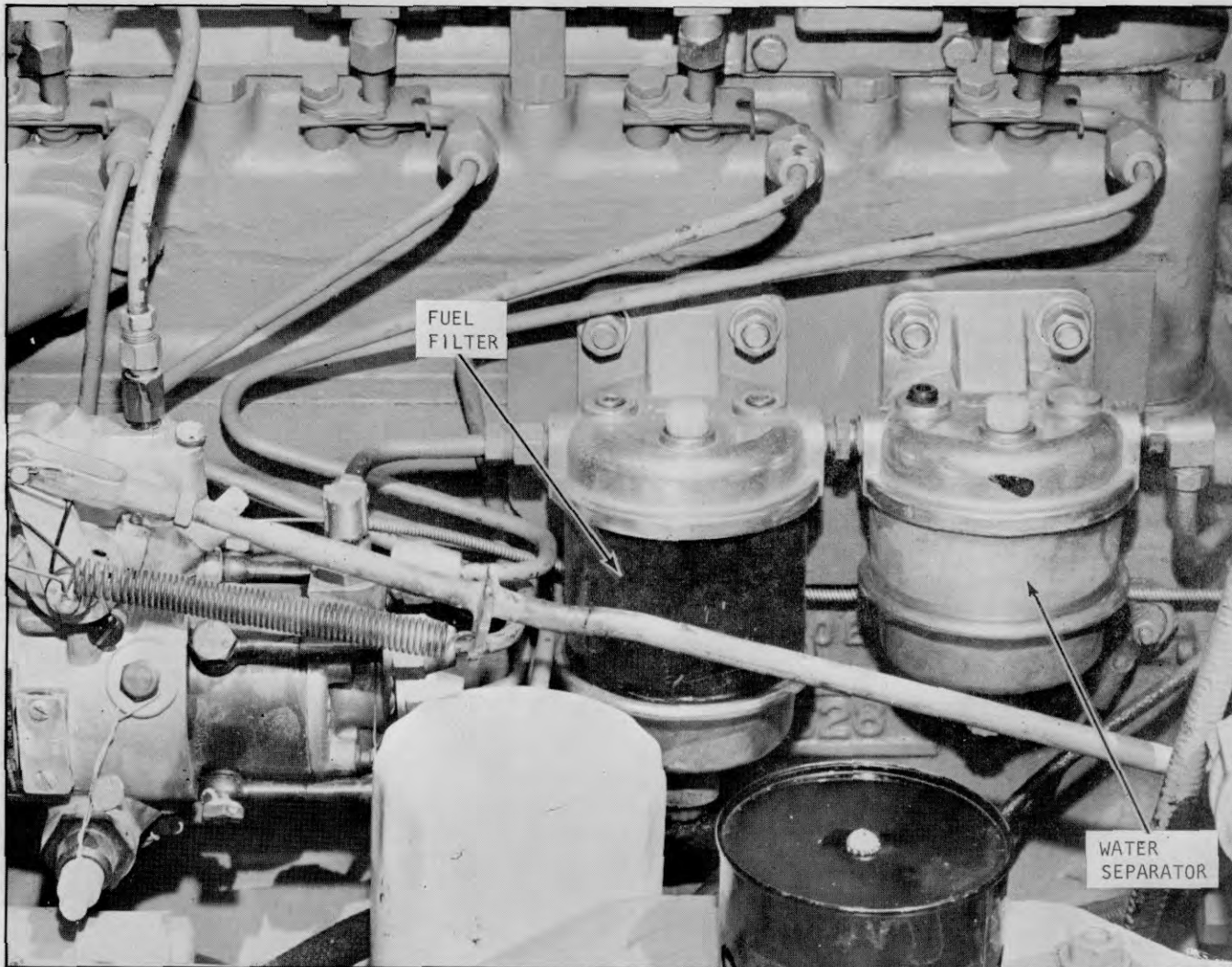
Plate 10196. Typical Fuel Filter
