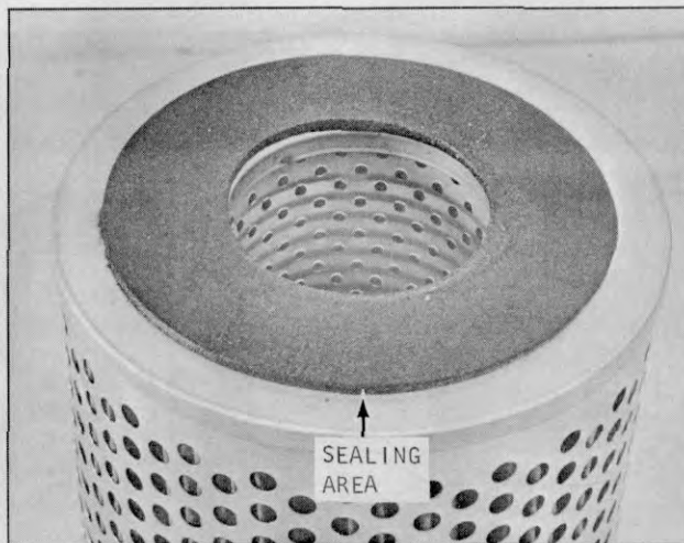
Plate 9741. Typical Filter Element
