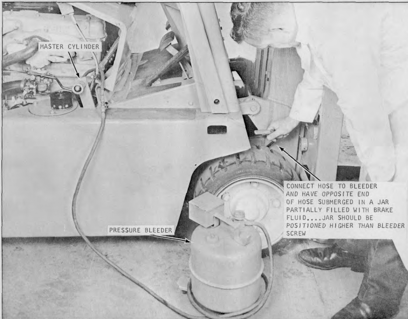
Plate 9791. Typical Pressure Bleeding
