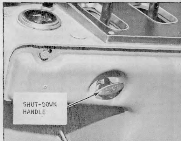
Plate 10178. Typical Shut-Down Handle
