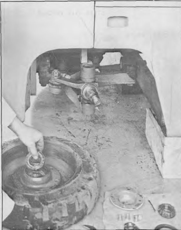
Plate 9768. Steer Wheel Bearings
