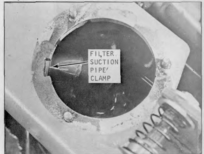
Plate 9622. Typical Hydraulic Filter Suction Pipe
