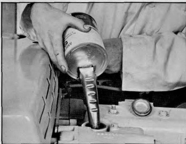
Plate 10188. Typical Crankcase Fill Procedure
