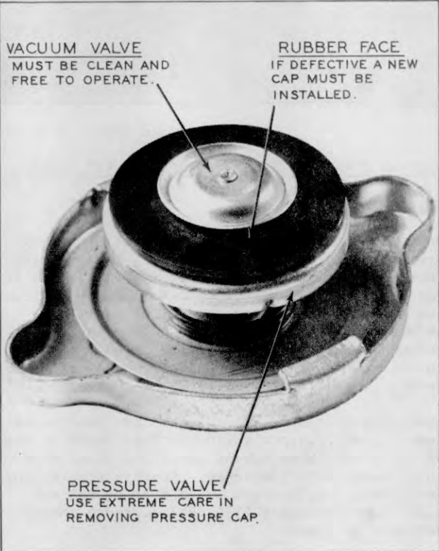
Plate 6459. Pressure Cap Gasket, Valve and Valve Gasket
