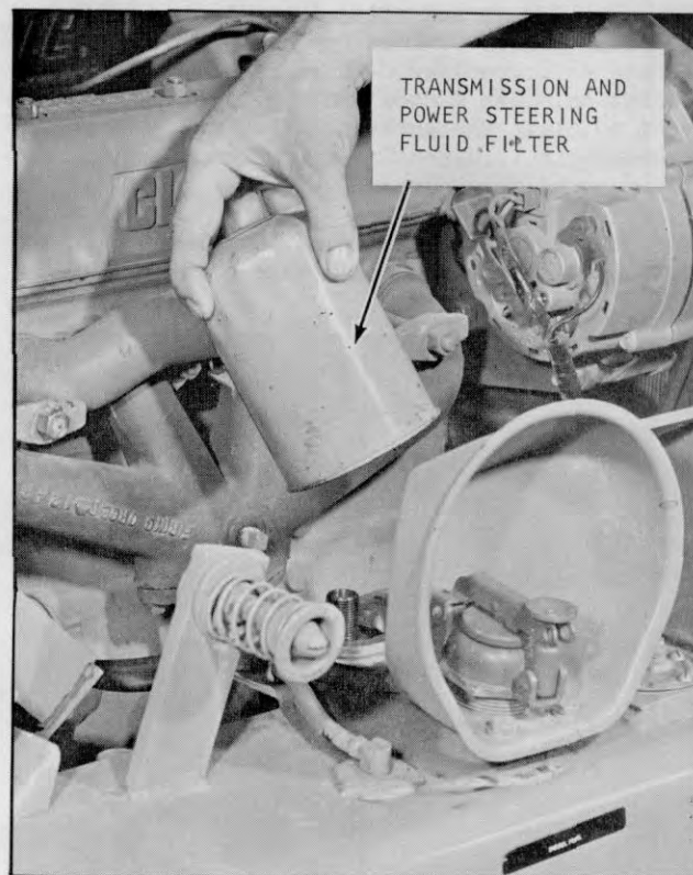
Plate 10183. Typical Transmission Filter
