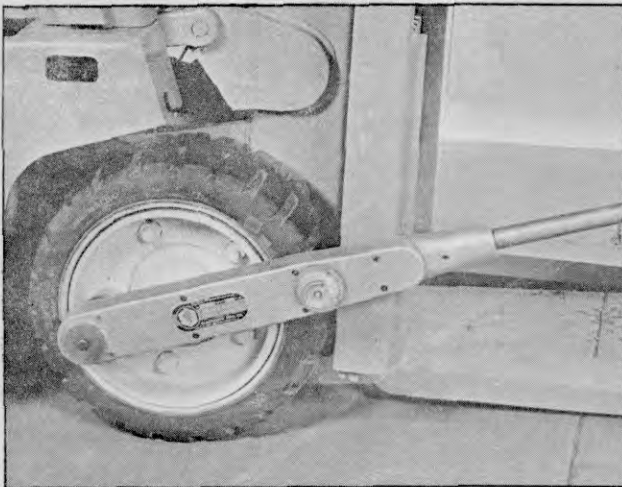
Plate 9852. Torque Drive Wheel Lug Nuts
