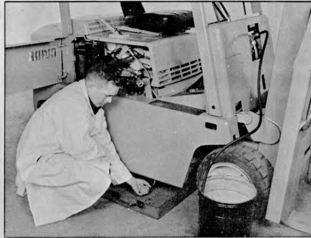
Plate 9794. Typical Sump Tank Drain
