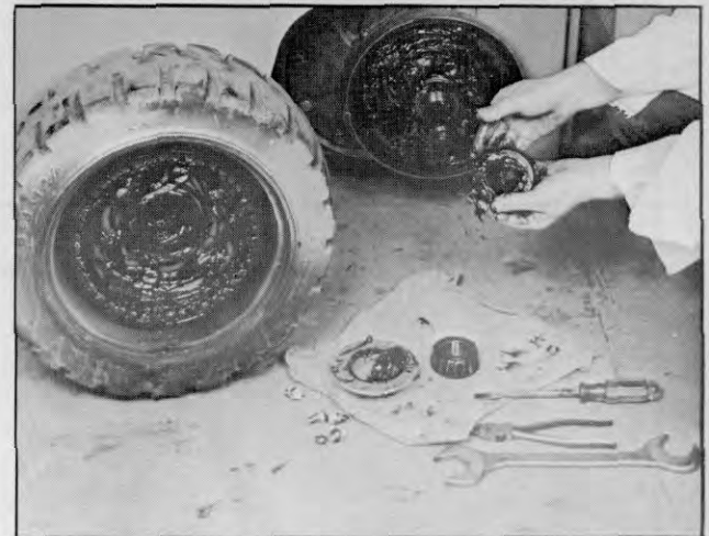
Plate 9775. Repack Axle End
