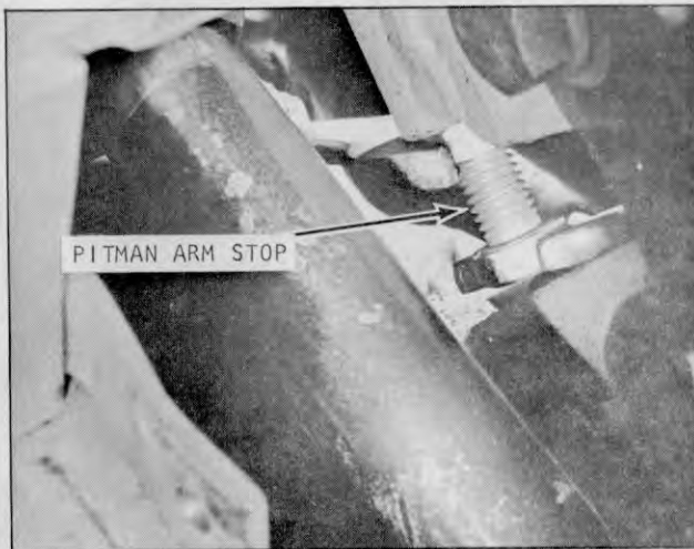
Plate 9771. Adjusting Pitman Arm Stops
