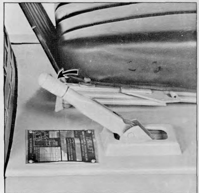
Plate 9781. Typical Parking Brake Lever
