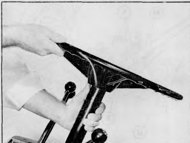
Plate 9843. Check Hand Wheel End Play
