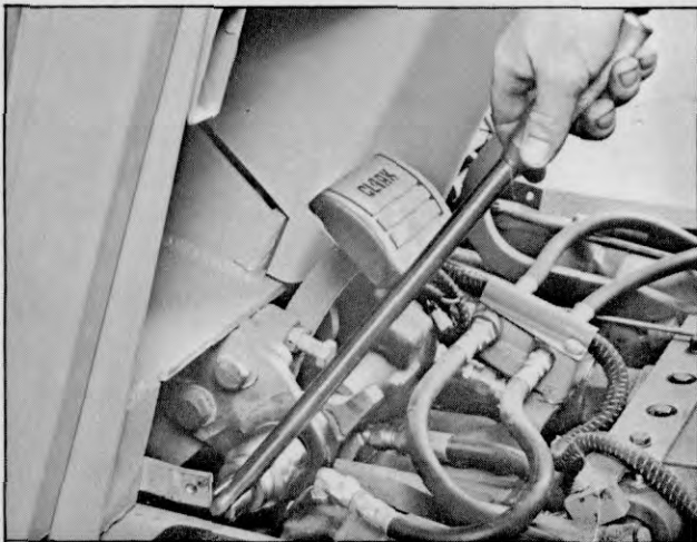
Plate 9848. Torque Pitman Arm Shaft Locknut
