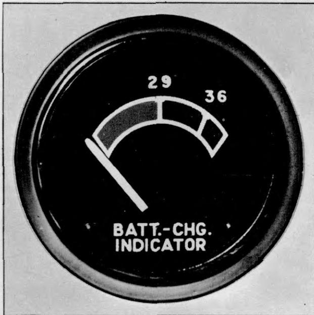
Plate 7388. Battery Charge Indicator
