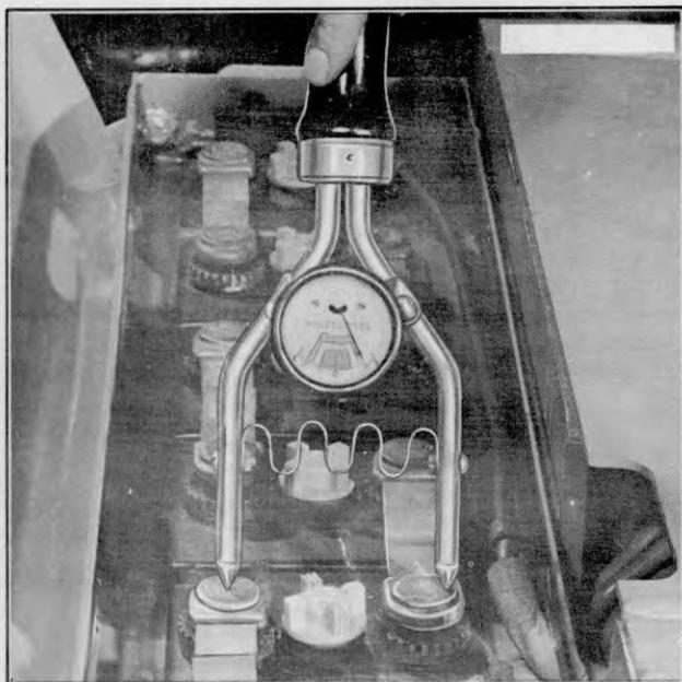
Plate 4008. Charge Test Fork Check
