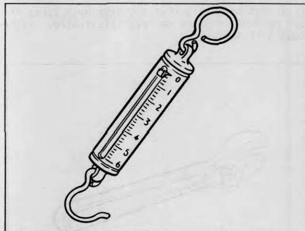
Plate 9679. Typical Instrument Type "T" - Chatillon Spring Tension Gage, Mfg. by Chatillon Inst. Co., New York, N.Y.
