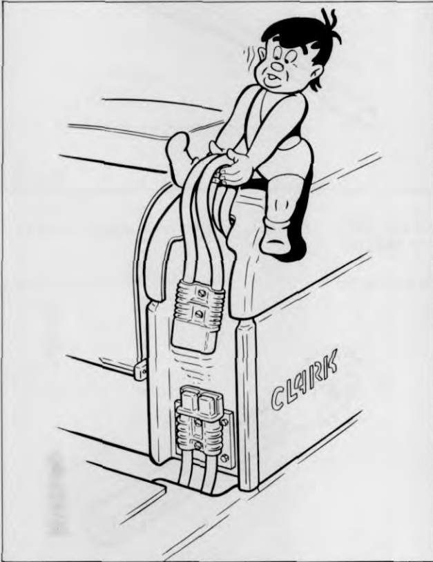
Plate 9688. "Typical" Battery Disconnect
