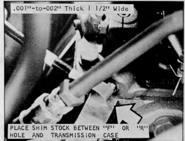
Figure 1705c. Install Shim Stock
