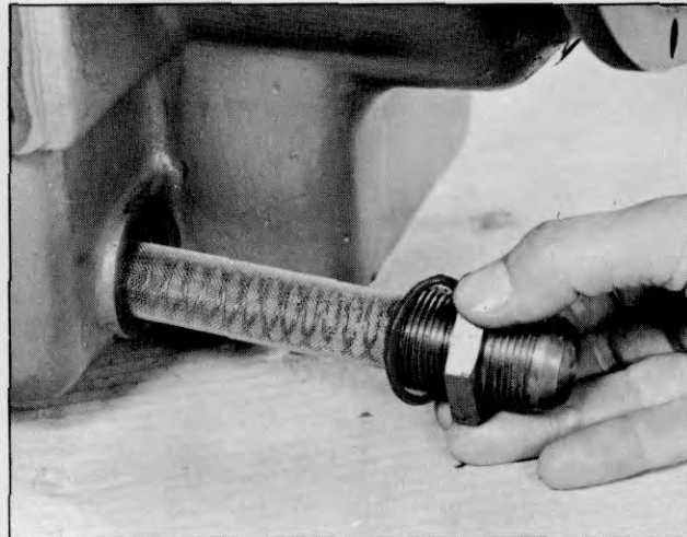
Plate 7235. Transmission Sump Screen
