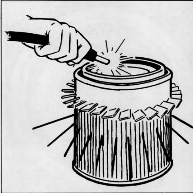
Plate 7173. Cleaning Dusty Element
