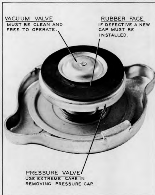
Plate 6459. Pressure Cap Gasket, Valve and Valve Gasket
