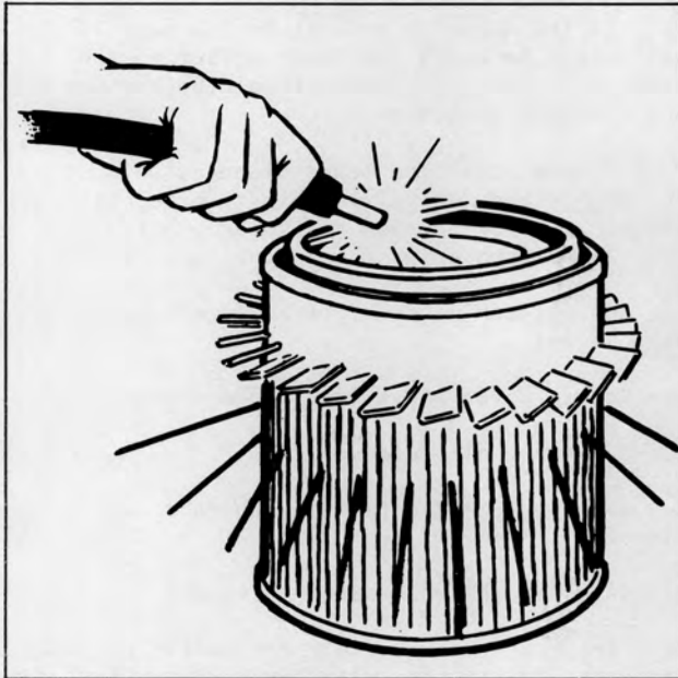
Plate 7173. Cleaning Dusty Element
