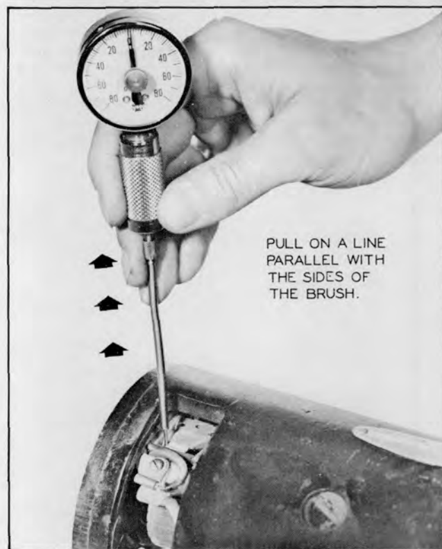
Plate 6450. Checking Brush Spring Tension
