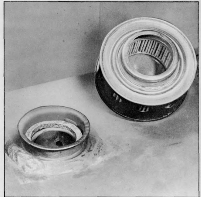
Plate 6682. Hydraulic Sump Tank & Sump Breather
