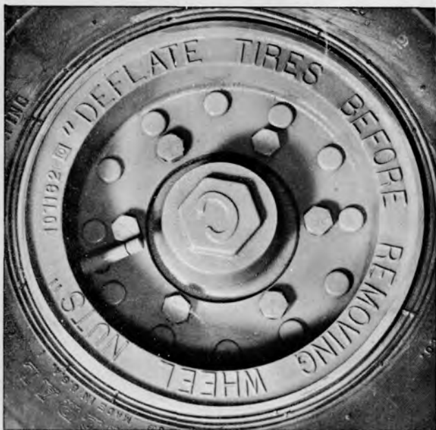
Plate 7613. Typical Wheel with Inner and Outer Halves
