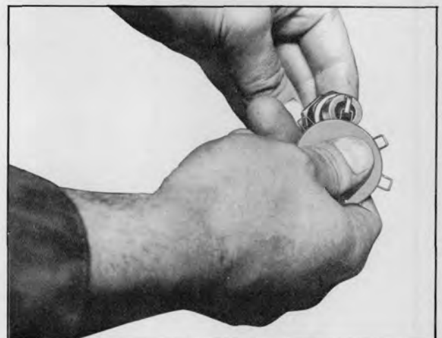
Plate 3278. Check Spark Plug Gap
