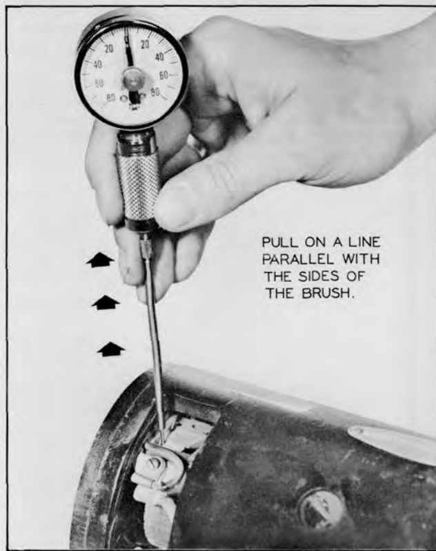
Plate 6450. Checking Brush Spring Tension
