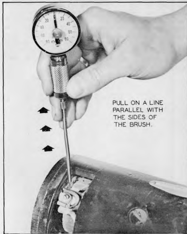
Plate 6450. Checking Brush Spring Tension
