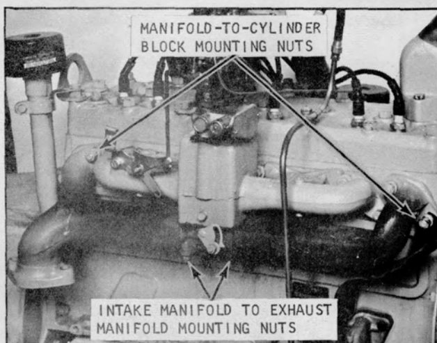
Plate 8452. Intake and Exhaust Manifolds
