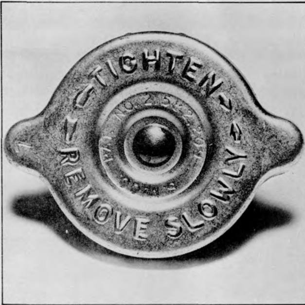
Plate 6458. Radiator Pressure Cap
