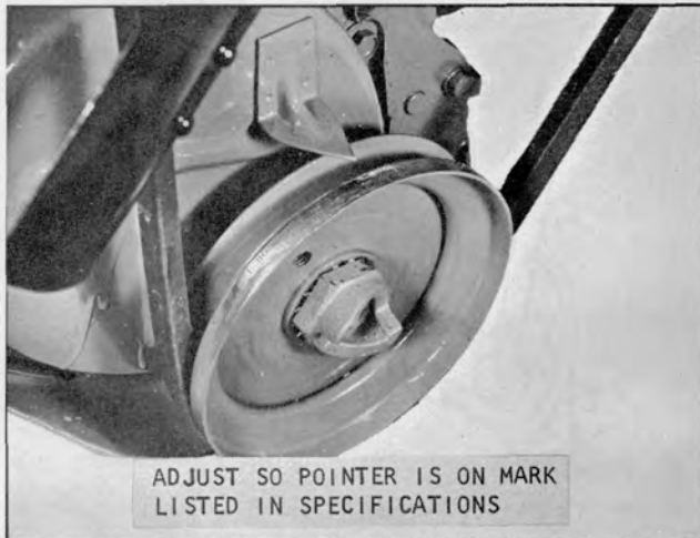
Plate 8462. Typical Timing Mark
