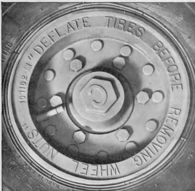
Plate 7613. Typical Wheel with Inner and Outer Halves
