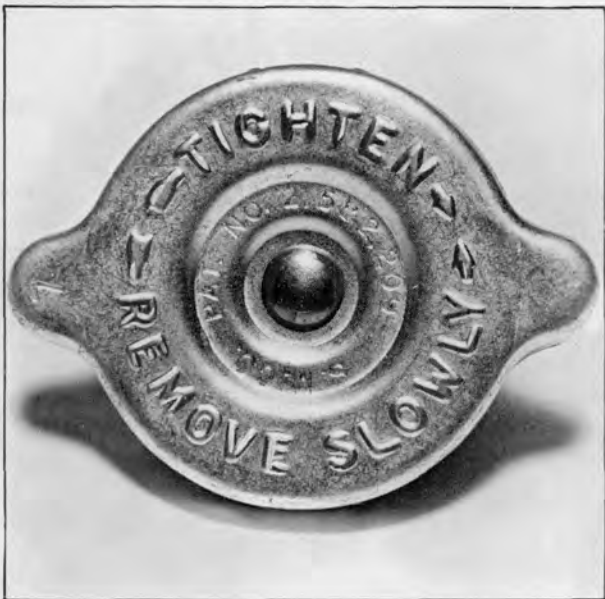
Plate 6458. Radiator Pressure Cap
