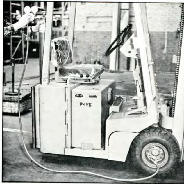
#11501. Shows Set-up Using Nitrogen Cylinder
