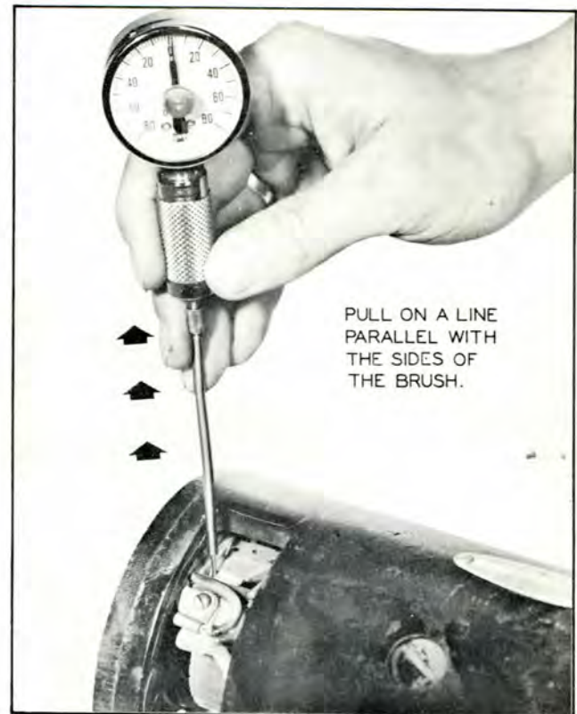
Plate 6450. Checking Brush Spring Tension
