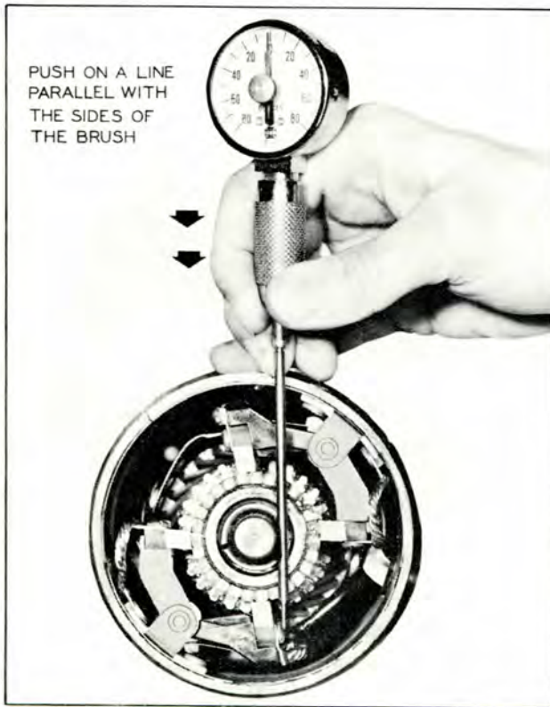
Plate 6449 Checking Brush Spring Tension
