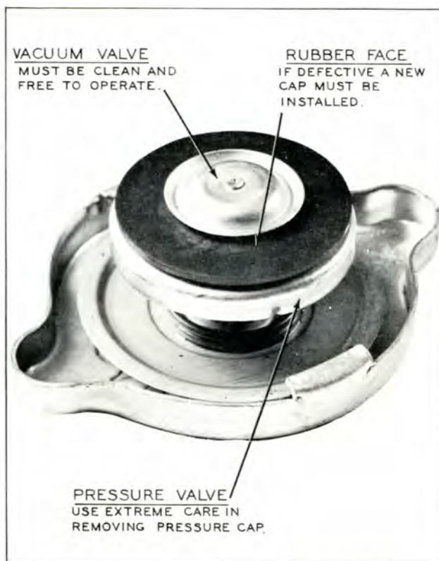
Plate 6459. Pressure Cap Gasket, Valve and Valve Gasket
