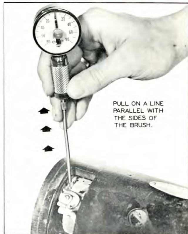
Plate 6450. Checking Brush Spring Tension
