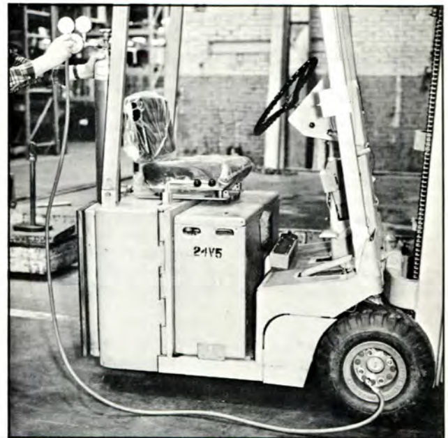
#11501. Shows Set-up Using Nitrogen Cylinder
