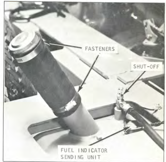
Plate 7427. Fuel Tank and Lines
