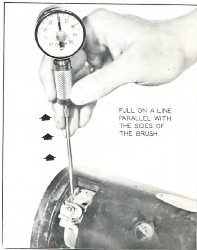
Plate 6450. Checking Brush Spring Tension
