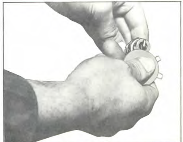
Plate- 3278. Check Spark Plug Gap
