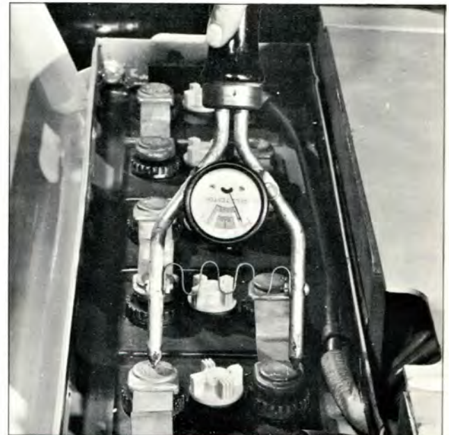
Plate 4008. Test Voltage of Cells
