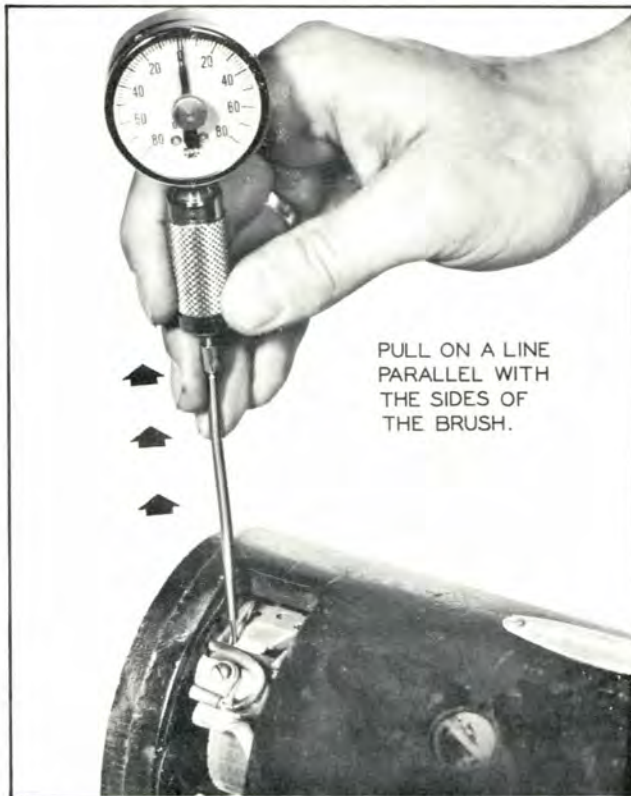
Plate 6450. Checking Brush Spring Tension
