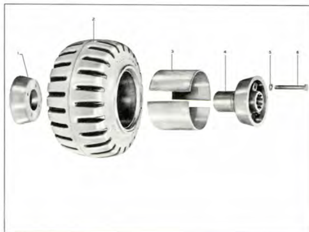
Plate 7343. Removable type Wheel and Tire Assy.
