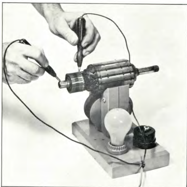
Plate 7222. Testing Armature for Shorted Coils FIELD COILS (ALL MOTORS)
