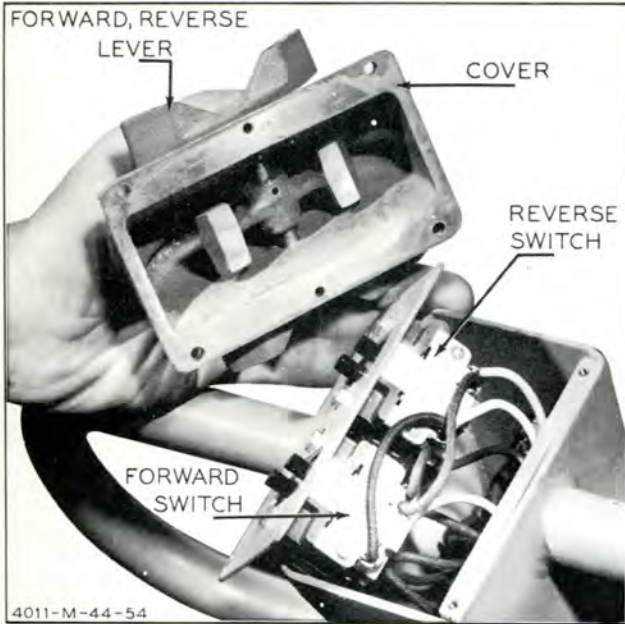
Plate 4011. Checking Forward and Reverse Switches
