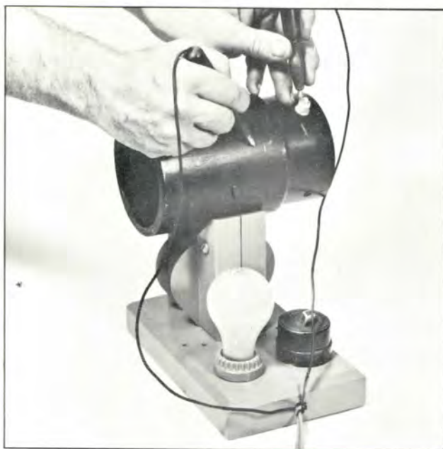
Plate 7223. Testing Field Coils for Grounds
